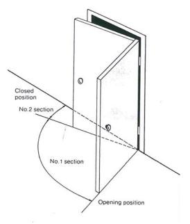
Adjusting Section of Closing Speed
